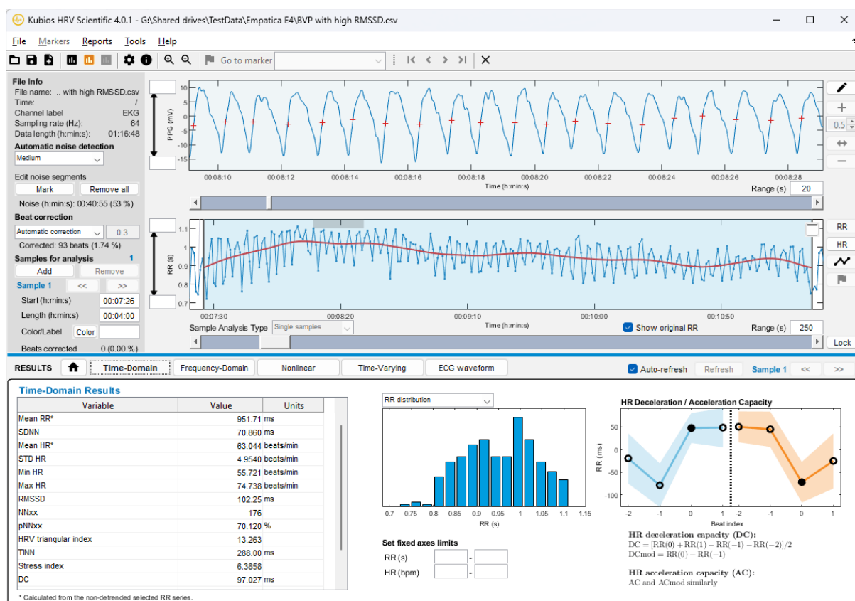
Figure 1: An example of high-quality PPG recording with periodic pulse waveforms of similar morphology. RR-interval series has no irregularities and all beat-to-beat intervals are physiologically realistic (in this case 0.7–1.1 sec).
